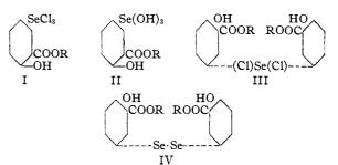
An attempt was made to prove the presence of hydroxyl groups in compounds of formula II by acetylation with acetyl chloride. The addition of acetyl chloride, however, regenerated the trichloride (formula I) and gave acetic acid as the other product. It has been shown by Nelson<sup>3</sup> and co-workers that the hydroxyl group para to selenium is not acetylated.
